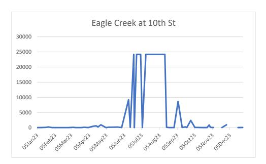
*E.coli* levels spiked at the 10<sup>th</sup> St site in June 2023. An investigation found a broken sanitary sewer pipe crossing the creek. Speedway Wastewater was notified in August, at which point the sewer was bypassed until repairs could be made.
