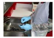
Ultrasonic cleaners work well to clean tools in hard-to-reach places and reduce the amount of time contaminated equipment is handled. Shop employers should check with the owner's manual to be sure the machine is cared for correctly.
